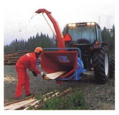
saplings, blocks, sawn surfaces and also frozen wood. The HP-21 can chip up to 170 mm size wood and branches. Operational noise is comparatively quiet, but it is a good idea to use ear protectors because of noise from the motor.
