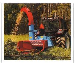
unpruned saplings, blocks, sawn surfaces and also frozen wood. The HP-25 can chip up to 230 mm size wood and branches. Operational noise is comparatively quiet, but it is a good idea to use ear protectors because of noise from the motor.
