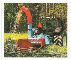
unpruned saplings, blocks, sawn surfaces and also frozen wood. The HP-28 can chip up to 280 mm size wood and branches. Operational noise is comparatively quiet, but it is a good idea to use ear protectors because of noise from the motor.
