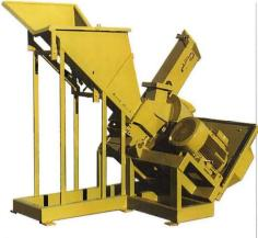
frozen. The wood is generally fed in using the chipper feed belt. The chipper wings blow the chips into the chip silo or on to a platform - up to 10 m away. If the chippers are placed inside as part of a production line they need separate noise insulation.
