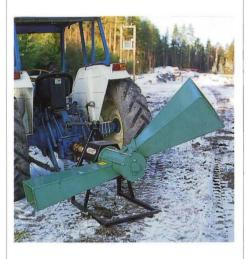
The LAIMET PS-10 is a tractor driven small chipper of remarkably simple construction. There are few parts that wear. It is reliable in operation and needs little maintenance.
